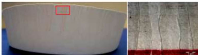
Figure 2. The image of shape with wrinkles and microscopic image of wrinkles
